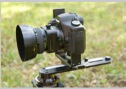
your lens the motions of Tilt, Swing and Shift. The lens itself has a much larger circle of coverage than that of a normal lens made for a 35 mm camera. This larger circle of coverage allows for the side-to-side and up-anddown movement of the lens. Advantages of a Tilt/Shift lens for panoramas:
